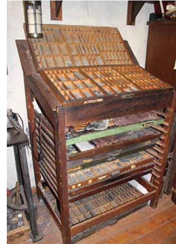
2. Printer's Type Stand with Cases
