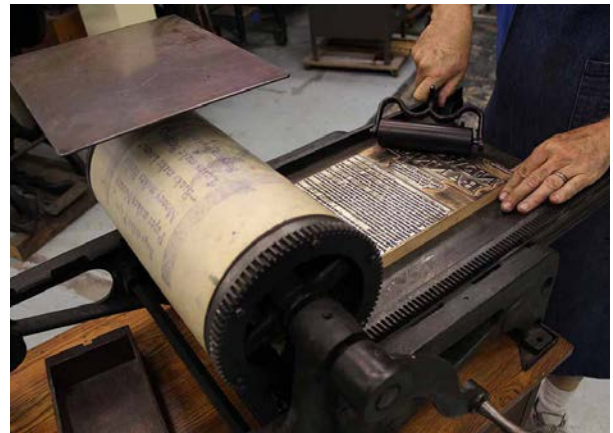
5.-A Inking Form POCO Printing Press
