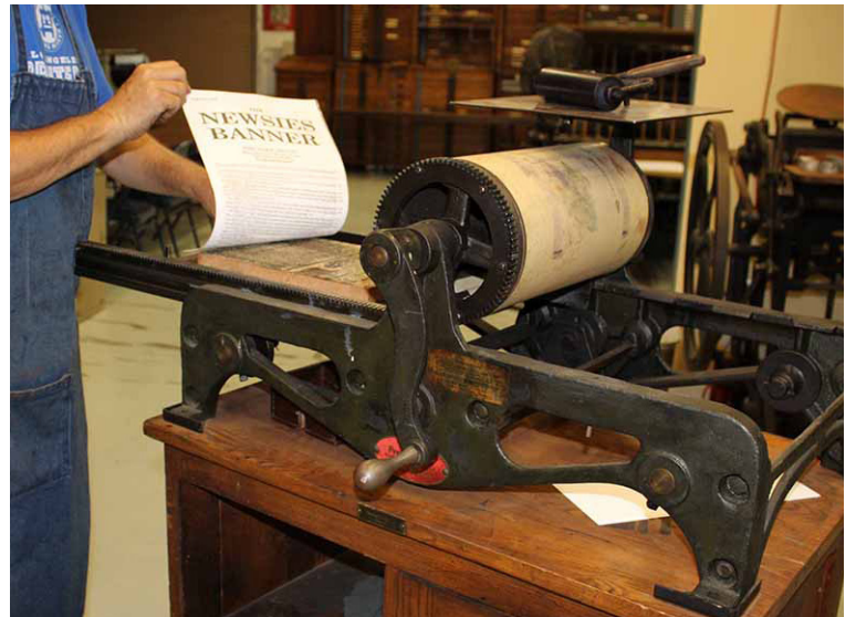
5-C Pulling Print on POCO Printing Press
