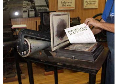
4-B Lowe Printing Press Pulling Print
